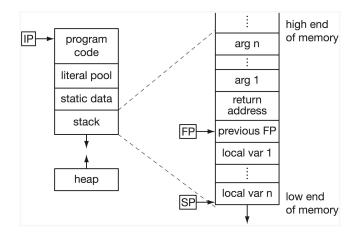
Fig. 1. Process memory organization and the stack layout.
