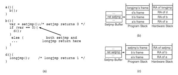
Fig. 3. Setjmp()/longjmp() example. (a) Code snippet, (b) program stack and hardware stack just before longjmp() returns, and (c) program stack and hardware stack just before setjmp() returns.
